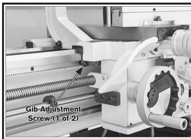
Figure 126. Front saddle gib adjustment screw.
